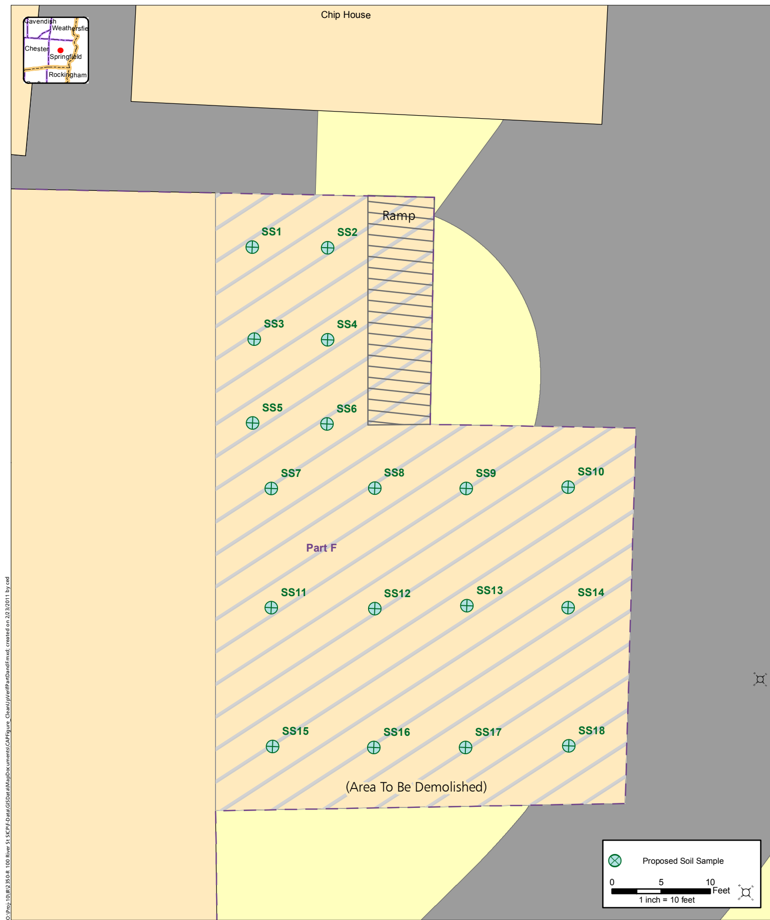
Figure 6: Proposed Clean Up Verification Sample Locations; Part D & F 100 River Street, Springfield, Vermont
